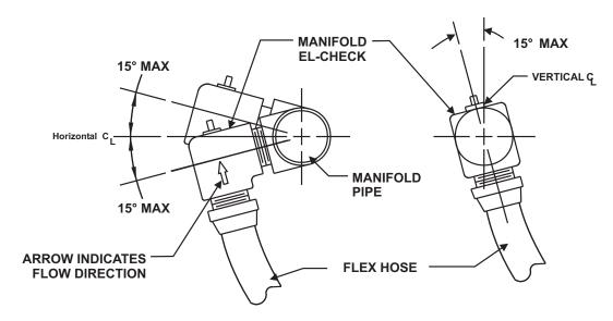
Note: Install El-Checks so that the arrow is in the direction as indicated.
